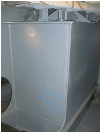
8. Plating of sea chests. Shell plating in way of overboard discharges as considered necessary by the attending surveyor.
