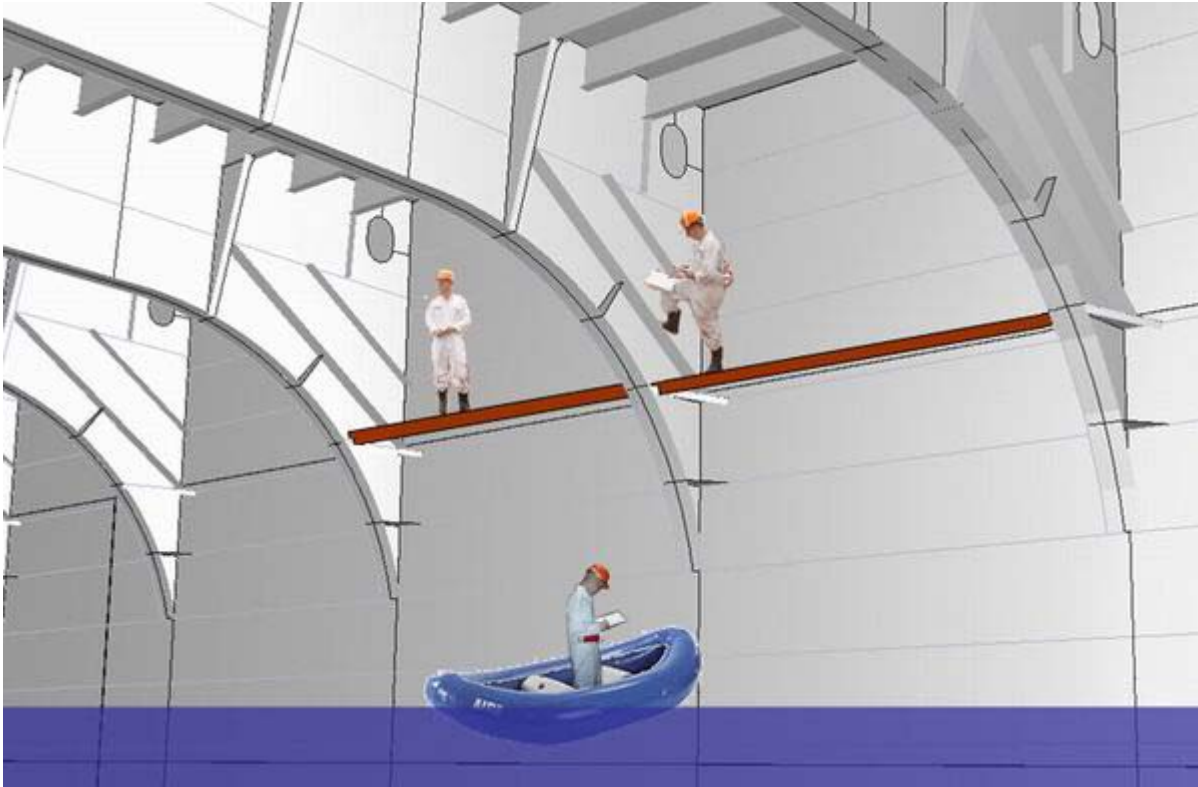
Fig. 4.4.4 Schematic illustration of how close-up may be achieved without rafting underneath deck. Temporary staging is placed between the flanges of the web frames. Tank is partly filled for safety reasons.
