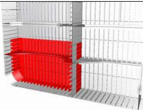
7. Lower part of one transverse bulkhead - in each remaining ballast tank. 8. Lower part of one transverse bulkhead - in a cargo oil wing tank.
